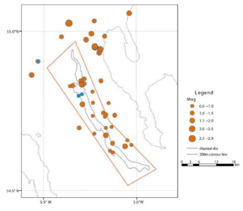
**Figure 4.8**: Locations and magnitude (Richter Scale ML) of underwater explosions in the Beaufort's Dyke area between 1992 and 2004 that were detected by the BGS seismograph network and are available in the BGS seismicity database. The blue circles show three explosive events identified during the BGS analyses that had not been previously attributed to the Beaufort's Dyke area. Source: BGS, 2005.
